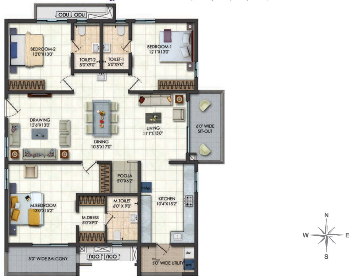
Carpet Area 1487 Sft | Wall Area 96 Sft | Balcony & Utility Area 242 Sft | Common Area 510 Sft
